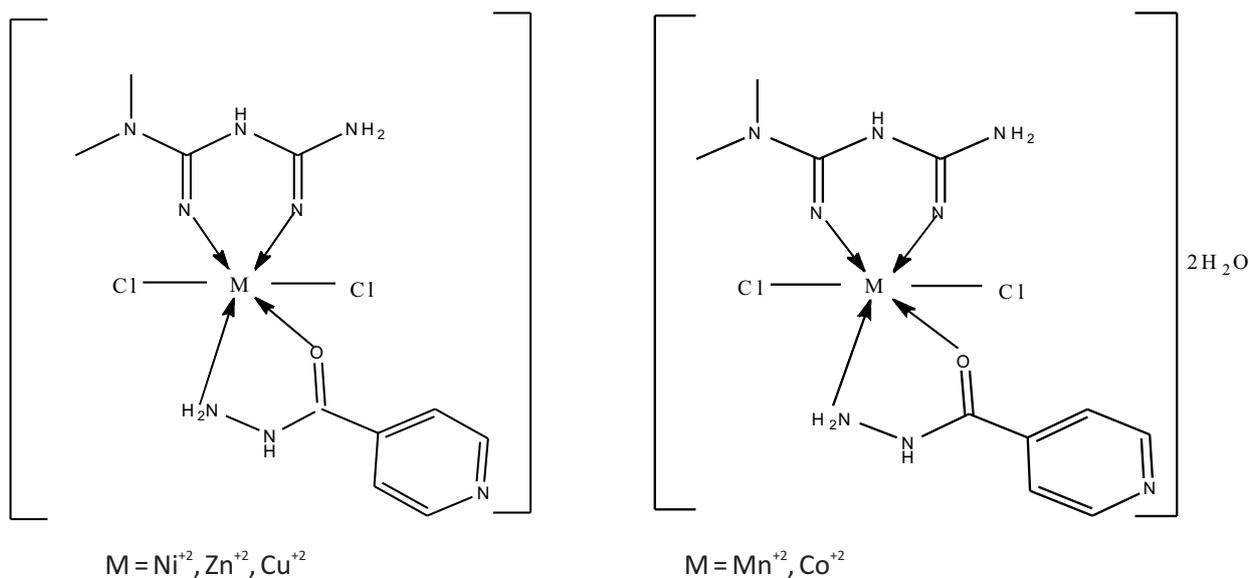
**Figure 3:** Proposed Structure of Mixed Ligand Metal Complexes of Metformin with Isoniazid
