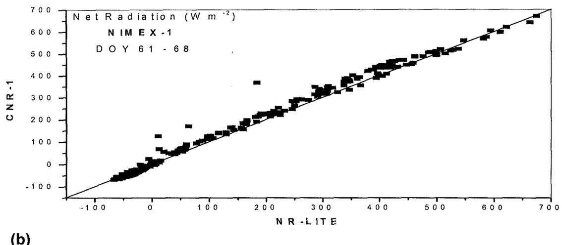
Fig. 9: Comparisons of (a) global and (b) net radiation as measured by SP-LITE and NR-LITE radiometers respectively with a reference net radiometer, CNR-1.
