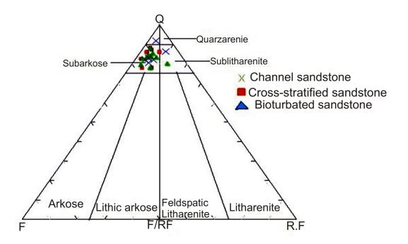
Fig. 4: QFR Triangular Classification Plot (Folk, 1974) for the Eze-Aku Sandstone Samples.
