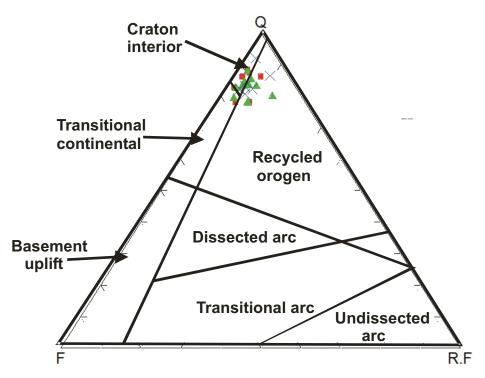
Fig. 8: QtFRF Ternary Diagram for the Eze-Aku Sandstone, after Dickinson et al. (1983)
