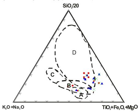
Figure 10: Plot of the Major Element Composition of the Eze-Aku Sandstone on the Tectonic Setting Discrimination Diagram of Kroonenberg (1994). A: Oceanic Island Arc; B: Continental Island Arc; C: Active Continental Margin; D: Passive Margin
