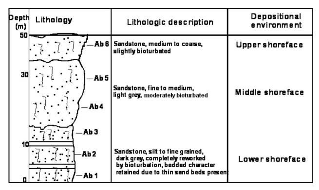
Fig. 2: Lithologic Succession of the Exposed Outcrop at Abini Quarry
