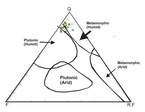
Fig. 6: The Effect of Source Rock on Composition of the Eze-Aku Sandstone using Suttner *et al.* (1981) Diagram
