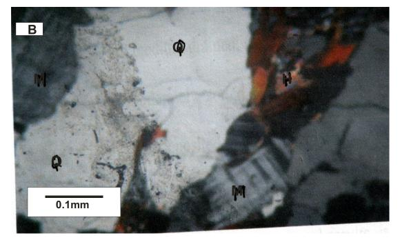
Fig. 3: A: Photomicrograph Showing Quartz Grains with Undulose Extinction (black Arrow) and Straight Extinction (white Arrow); B: Photomicrograph under a Cross Nicols Light Showing Quartz (q), Microcline Feldspar (m), and Heavy Minerals (h)
