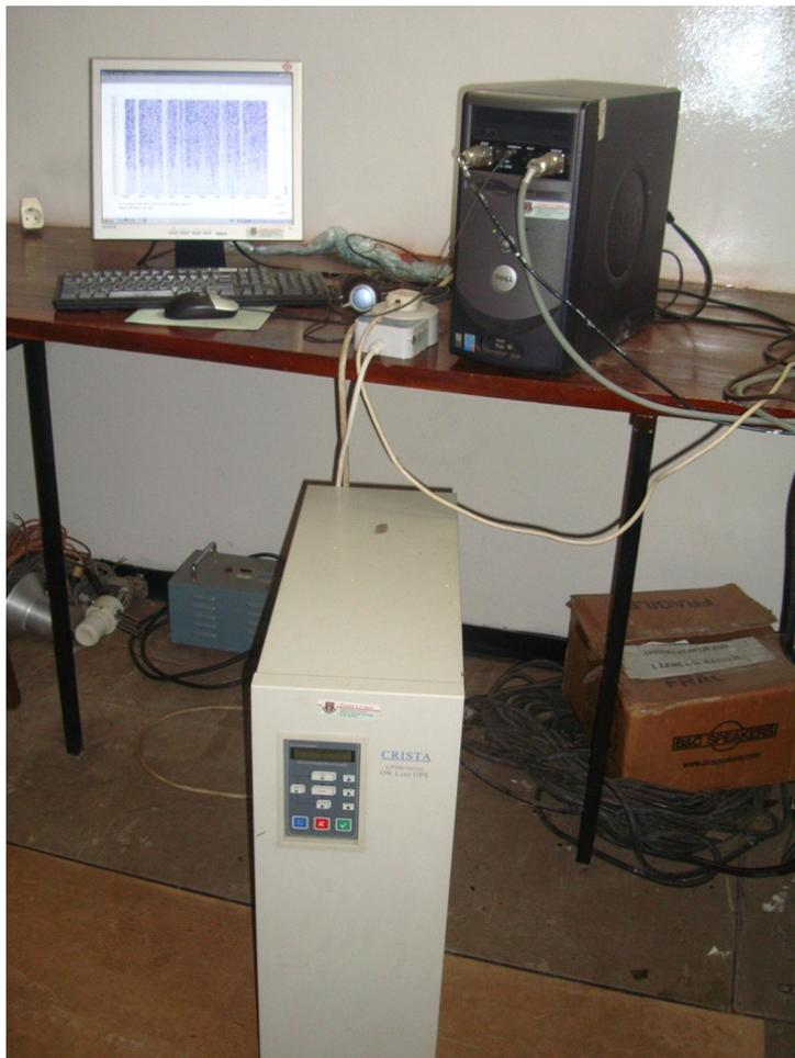
Fig.2: The Indoor Desktop Computer that Controls the Sodar Antenna with the UPS; the Monitor Displays the 10 Minutes Averages of Wind Profile Measured by the System, the Gaps Indicates Periods of Power Outage.
