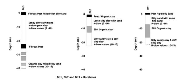
Figure 2: Borehole Lithologic logs with Standard Penetration Test Results
