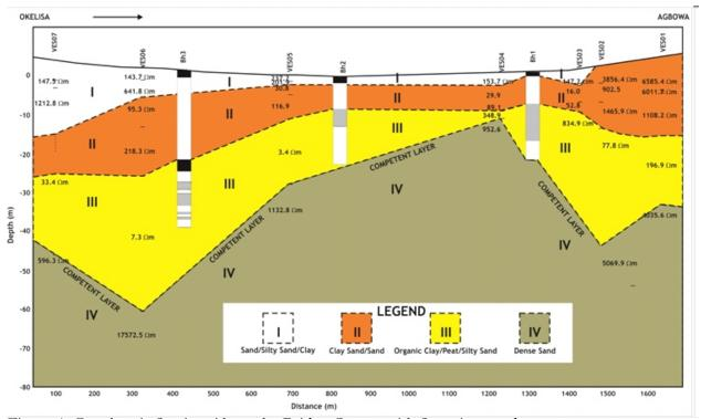
Figure 4: Geoelectric Section Along the Bridge Course with Superimposed Borehole Lithological Logs
