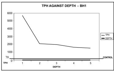
Fig. 5a: Graph of TPH against Depth of Borehole 1
