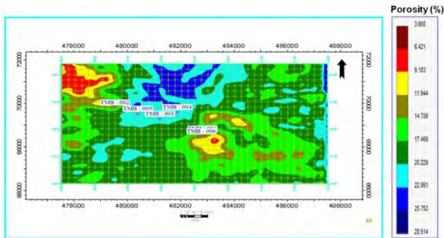
Figure 11: Horizon Based RMS Porosity Map of TMST4 Showing the Sand-Facies Distribution (Produced with Petrel Software, 2010).
