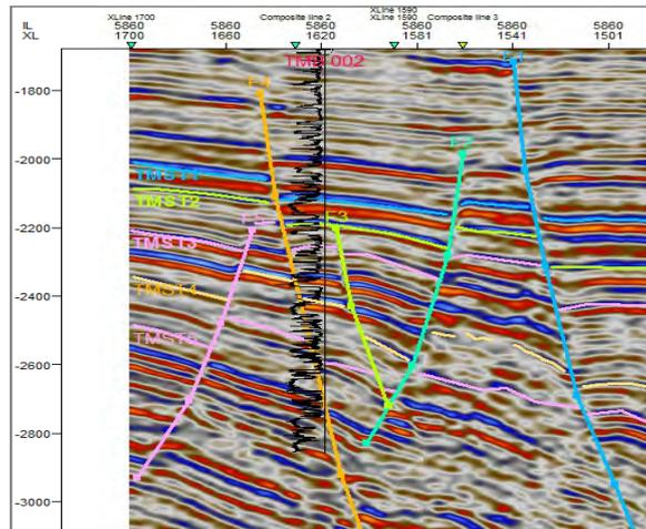
Figure 6: Seismic Section of Inline 5860 Showing the Fault Segments and Interpreted Horizons (Produced with Petrel Software, 2010).
