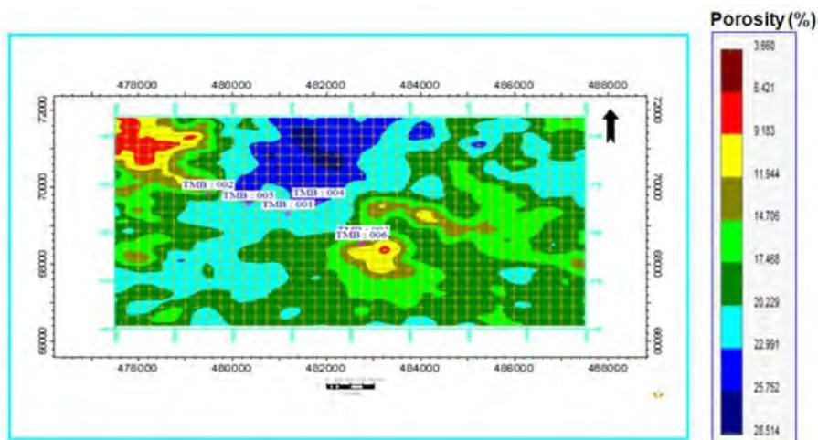
Figure 12: Horizon Based RMS Porosity Map of TMST5 Showing the Sand-Facies Distribution (Produced with Petrel Software, 2010).
