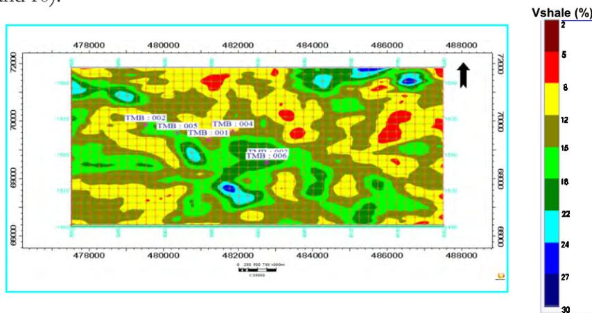
Figure 9: Horizon Based RMS  $V_{shale}$  Map of TMST4 Showing the Sand-Facies Distribution (Produced with Petrel Software, 2010).
