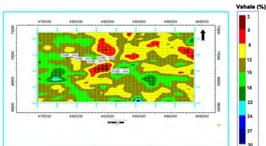
Figure 10: Horizon Based RMS  $V_{shale}$  Map of TMST5 Showing the Sand-Facies Distribution (Produced with Petrel Software, 2010).
