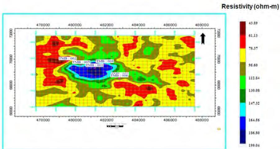
Figure 14: Horizon Based RMS Resistivity Map of TMST5 Showing the Sand-Facies Distribution(Produced with Petrel Software, 2010).
