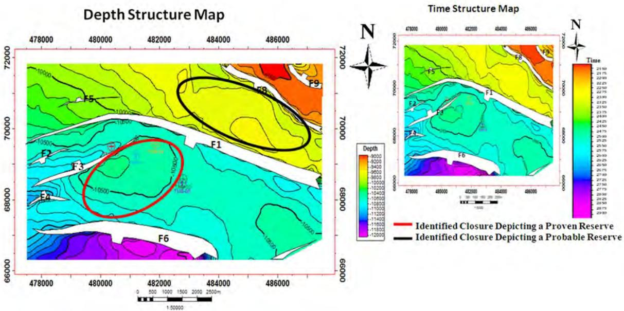
Figure 8: Depth and Time Structure Maps of Horizon TMST5 Showing Identified Fault Polygons and Closures(Produced with Petrel Software, 2010)
