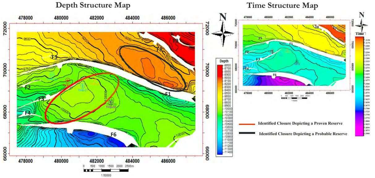
Figure 7: Depth and Time Structure Maps of Horizon TMST4 Showing Identified Fault Polygons and Closures(Produced with Petrel Software, 2010).
