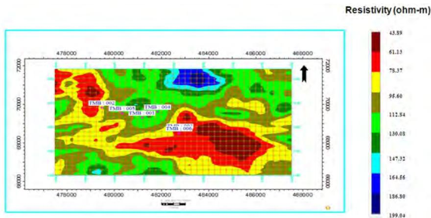
Figure 13: Horizon Based RMS Resistivity Map of TMST4 Showing the Sand-Facies Distribution(Produced with Petrel Software, 2010).
