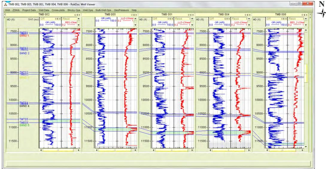
Figure 4: Well Correlation of the Identified Reservoir Sands and their Lateral Continuity (Produced with RokDoc Software, Version 6.1.4)
