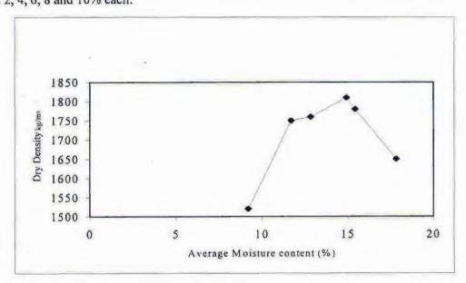
Fig.1: Compaction curve for 100% (unstabilized) soil sample
