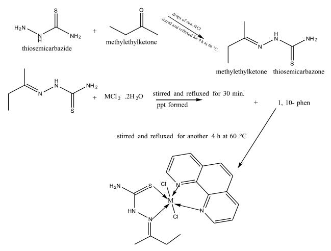
Scheme (1) : Synthetic Preparation of the mixed-ligand Complexes. [M(MEKT)(phen)Cl<sub>2</sub>]
