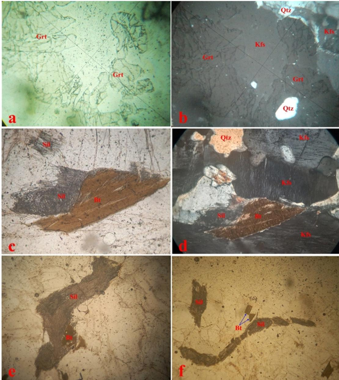
**Figure 3:** Photomicrographs showing: (a) porphyroblasts of garnet with numerous fractures, PPL (b) porphyroblasts of garnet (Grt) with inclusions of quartz (Qtz), surrounded by K-feldspar. XPL (c) fibrolitic sillimanite (Sil) at the edges of brownish biotite (Bt), PPL (d) K-feldspar mantling biotite (Bt), sillimanite (Sil) and quartz (Qtz), PPL (e) folded trails of sillimanite (Sil), PPL (f) fibrolitic sillimanite (Sil) mimicking foliation left by biotite (Bt), PPL
