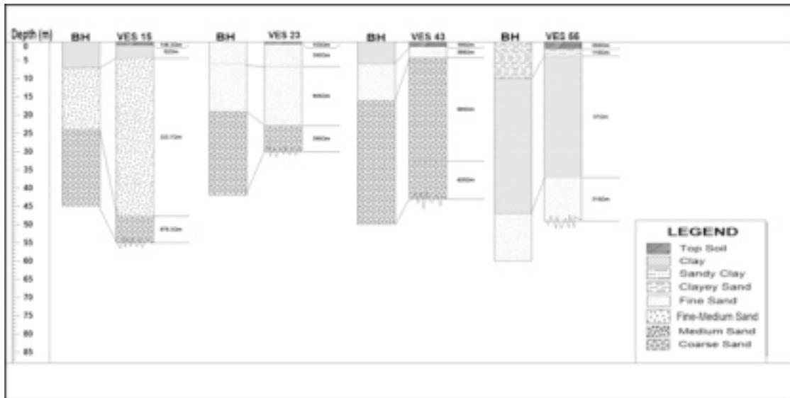
**Figure 4:** Geoelectric section for Ughoton, Ekakpamre, Uvwiamuge and Egbeleku.
