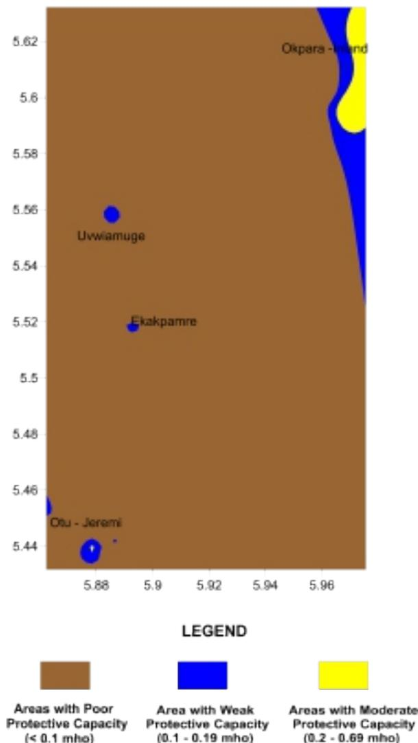
**Figure 6:** Vulnerability maps of Okpara-Inland, Uvwiamuge, Ekakpamre, and Otu-Jeremi based on longitudinal conductance (LC).
