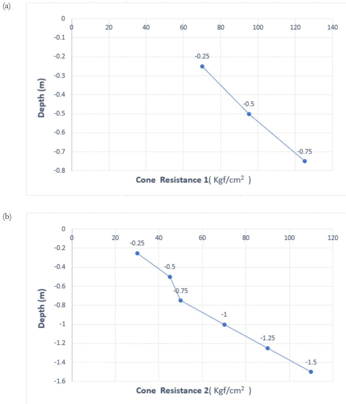
**Figure 8:** Cone resistance on (a) CPT 1 and (b) CPT 2.
