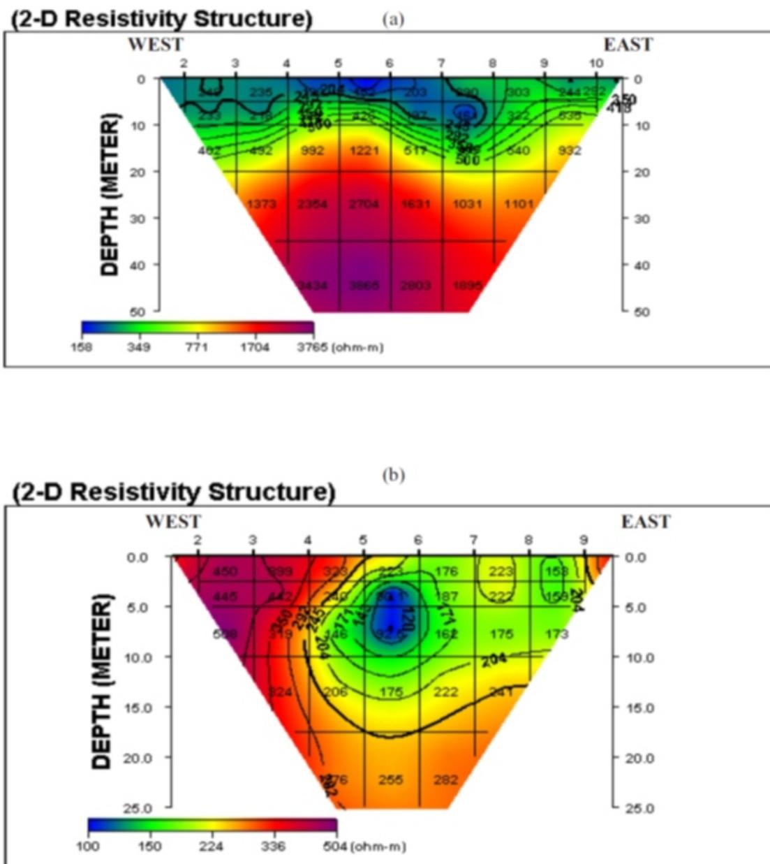
Figure 6: 2D resistivity structure along (a) Traverse 1, (b) Traverse 3.
