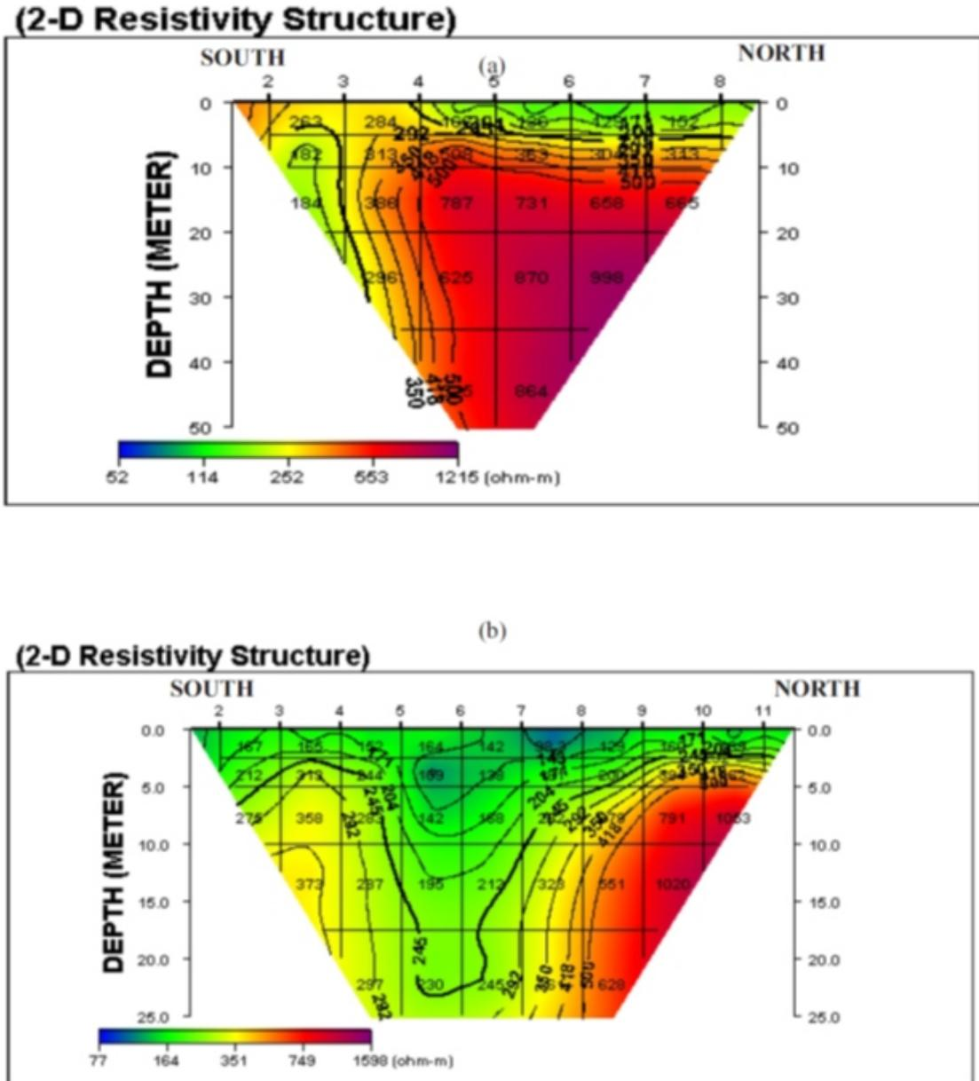
Figure 7: 2D resistivity structure along (a) Traverse 2, (b) Traverse 4.
