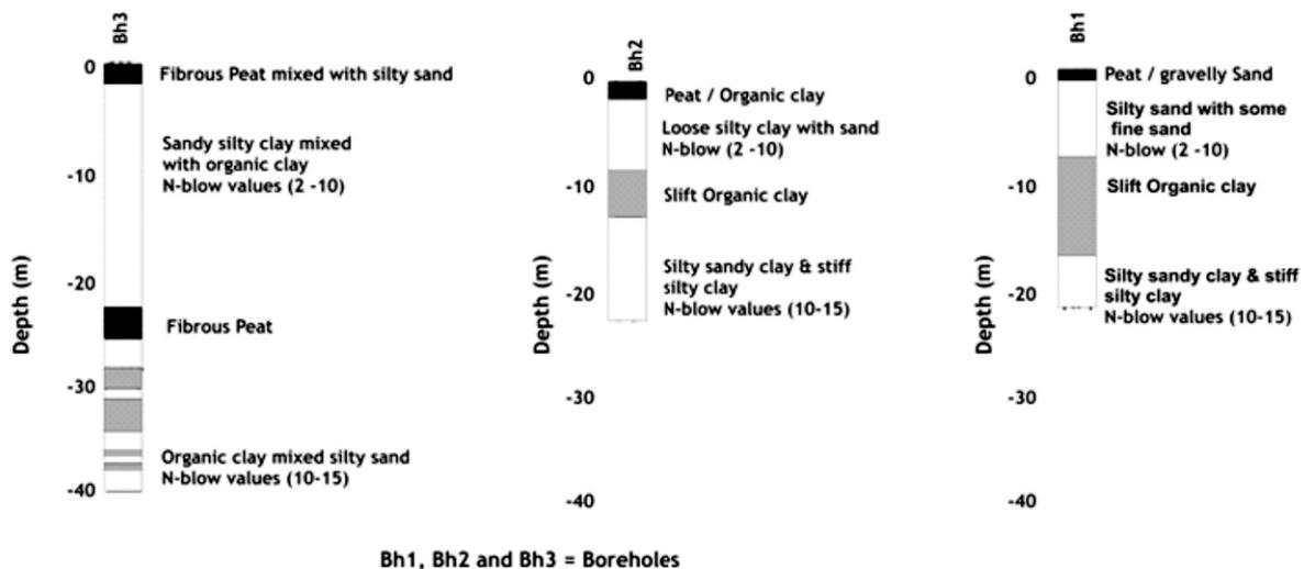
Figure 2: Borehole Lithologic logs with Standard Penetration Test Results
