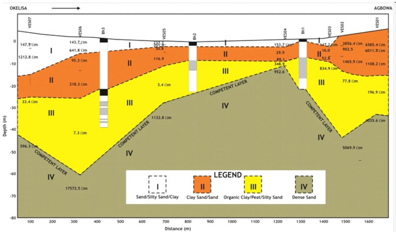
Figure 4: Geoelectric Section Along the Bridge Course with Superimposed Borehole Lithological Logs
