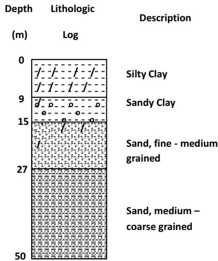
Fig. 5: Isaka Borehole I Log
