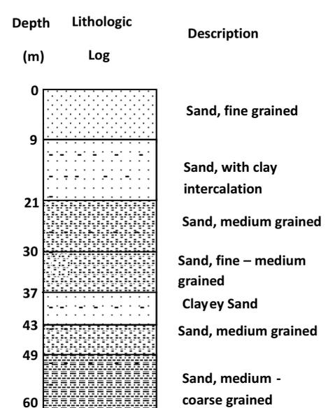
Fig. 7: Ogbogbo Borehole Log
