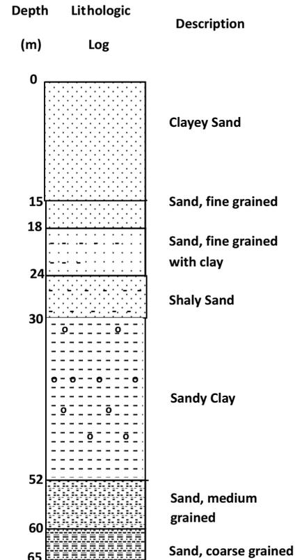
Fig.10: ATC Road Borehole Log
