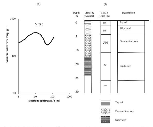
Fig. 2 (a) VES (VES 3) Curve and (b) Correlation of the VES Interpretation Results with the Lithology of the nearest Borehole
