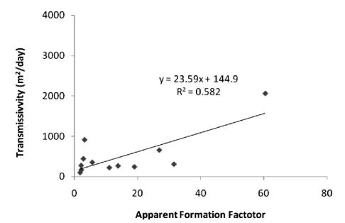
Fig.5. Relationship Between Transmissivity and Apparent Formation Factor
