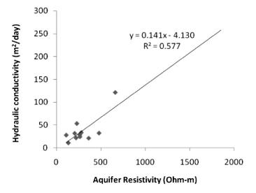
Fig.7. Relation Between Hydraulic Conductivity and Resistivity
