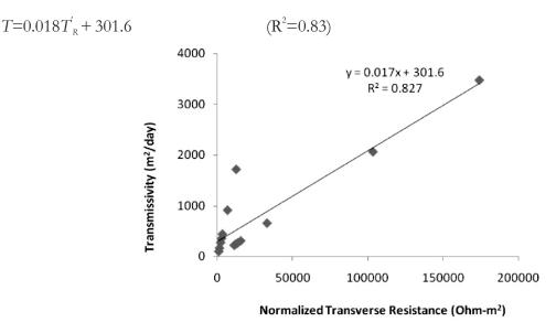
Fig. 6. Relation Between Transmissivity and Modified Transverse Resistance
