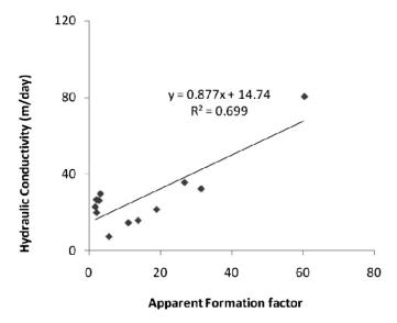
Fig. 4. Relation Between Hydraulic Conductivity and Apparent Formation Factor
