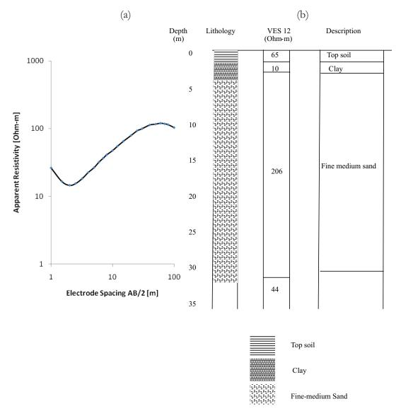
Fig. 3 (a) VES (VES 12) Curve and (b) Correlation of the VES (VES 12) Interpretation Results with the Lithology of the nearest Borehole.
