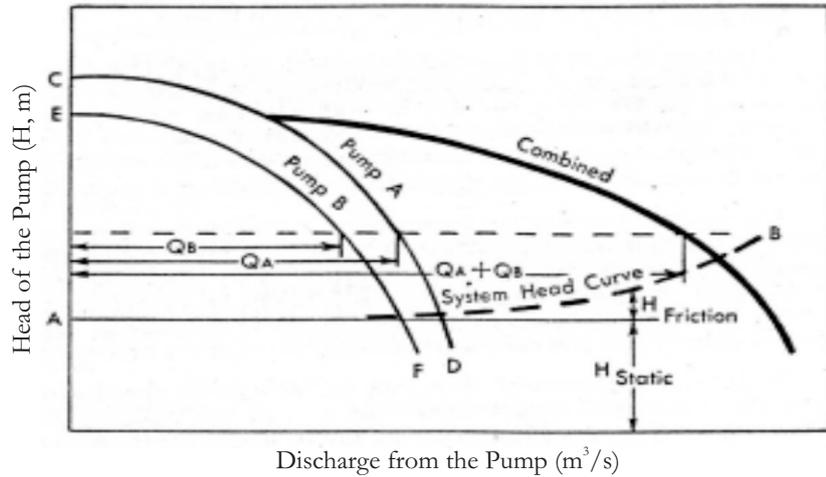
Figure 8a: Head Capacity Curves of Pumps Operating in Parallel (Source: Fairbank, 1965)
