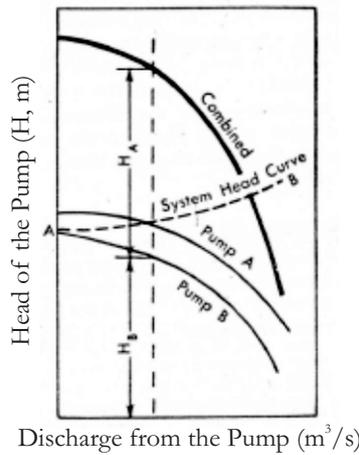
Figure 8b: Head Capacity Curves of Pumps Operating in Series (Source: Fairbank, 1965)
