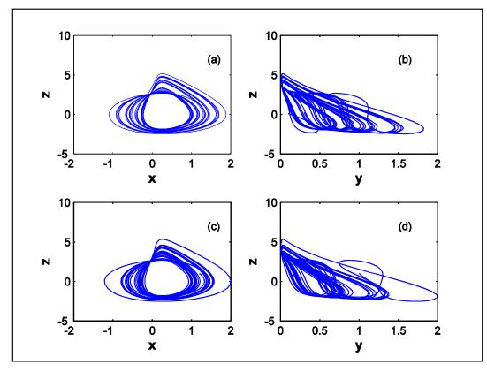
Figure 2: Phase portrait of chaotic attractor for initial conditions 1.0, 0.1, 0.1 ((a) and (b)) and for initial conditions 1.2, 1, 1 ((c) and (d))
