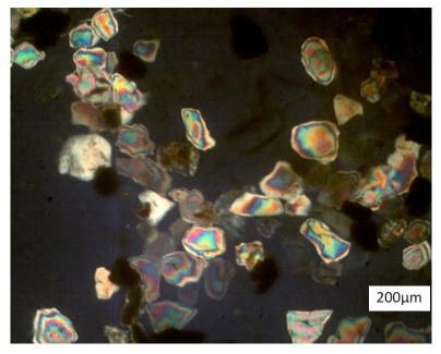
Fig.11: Photomicrograph of Heavy Minerals in xpl, Showing Zircon Grains, mostly Sub-angular to Angular.
