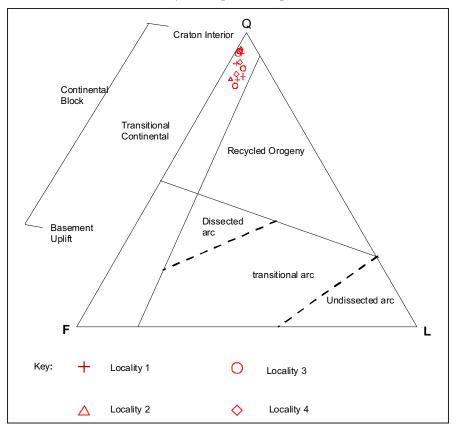
Fig 12: Ternary Diagram Showing Plot of the various Sandstone Clasts (Dikinson et al., 1983)
