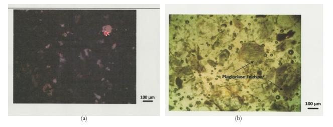
Fig.9: Photomicrograph of Sandstone from Felele Showing (a) Subhedral/anhedral quartz(Qz) in Xpl. (b) Sandstone in XplShowingPlagioclase feldspar grains
