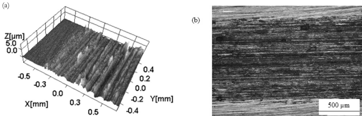
Fig. 9. (a) 3-D optical profile and (b) optical micrograph of flat sample for a typical 304L stainless steel-Al (2017) alloy pair after test
