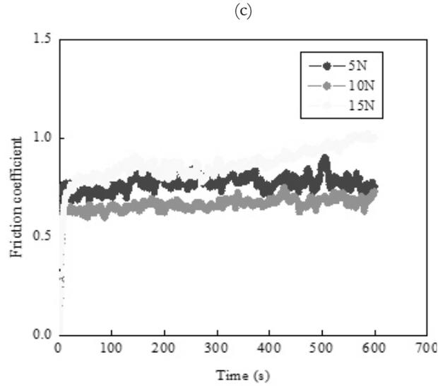
**Fig. 5.** Friction behavior under different loads for (a) 304L stainless steel-440C stainless steel (b) 304L stainless steel-Al alloy (2017) (c) 304L stainless steel-bronze pair.
