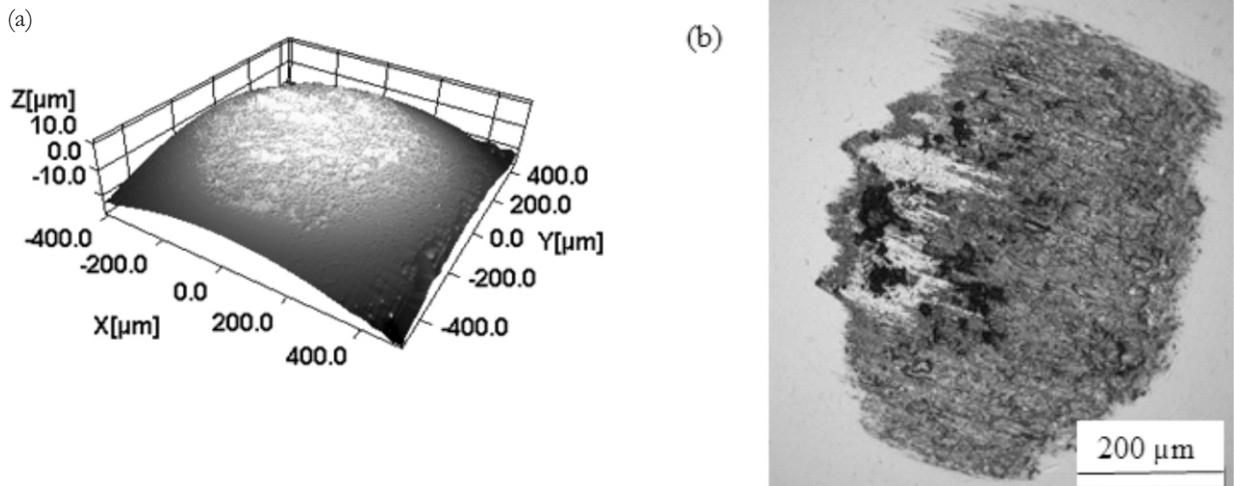
**Fig. 6.** (a) A typical 3-D optical profile (b) and the optical micrograph of the 440C stainless steel ball after the friction test.
