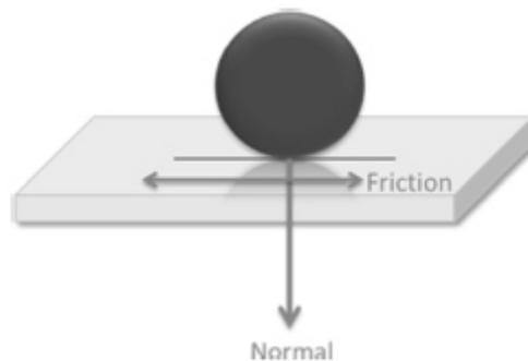
**Fig. 3.** Schematic diagram of ball-on-flat contact configuration under reciprocating sliding.
