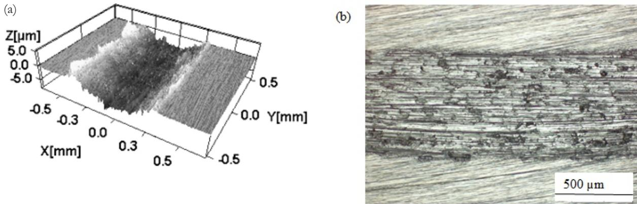
**Fig. 7.** (a) 3-D optical profile and (b) optical micrograph of flat sample for a typical AISI 304L stainless steel-440C stainless steel pair after test
