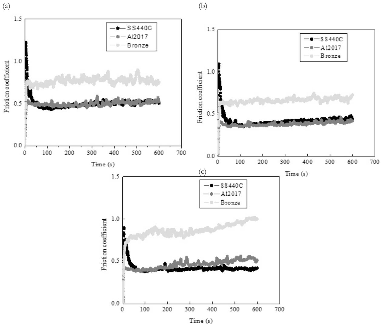
**Fig. 4.** Friction coefficient as a function of test duration at (a) 5 N (b) 10 N (c) 15 N for the pairs.
