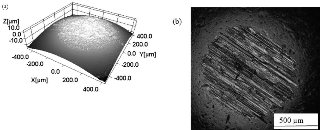
**Fig. 8.** (a) 3-D optical profile and (b) optical micrograph of bronze ball sample after friction test.
