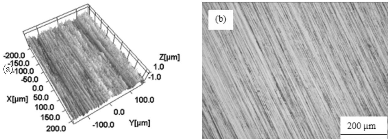
Fig. 1 (a) 3-D optical profile (b) optical micrograph of 304L stainless steel.
