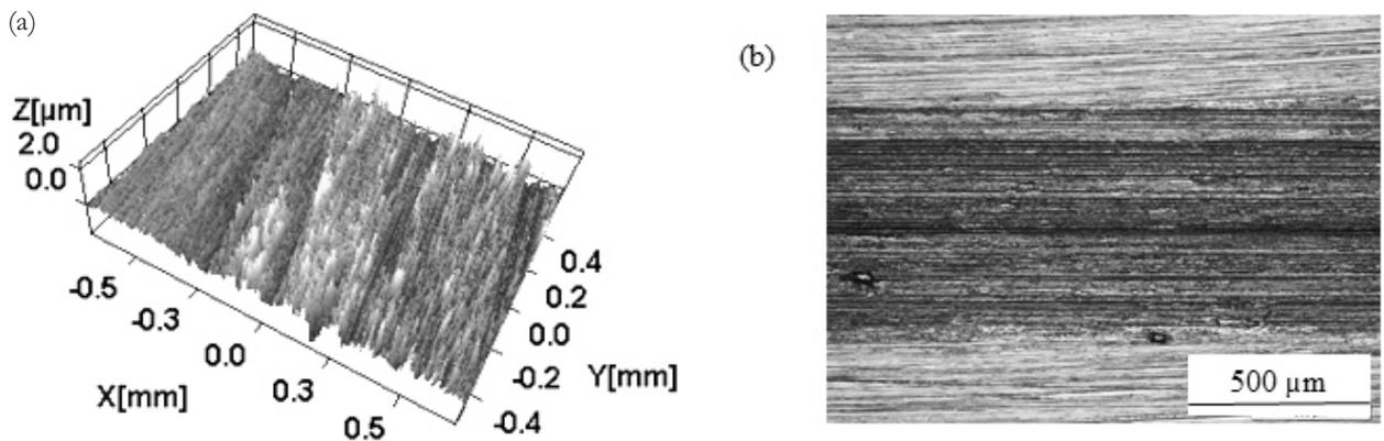
Fig. 10. (a) 3-D optical profile and (b) optical micrograph of flat sample for a typical 304L stainless steel-bronze pair after test
