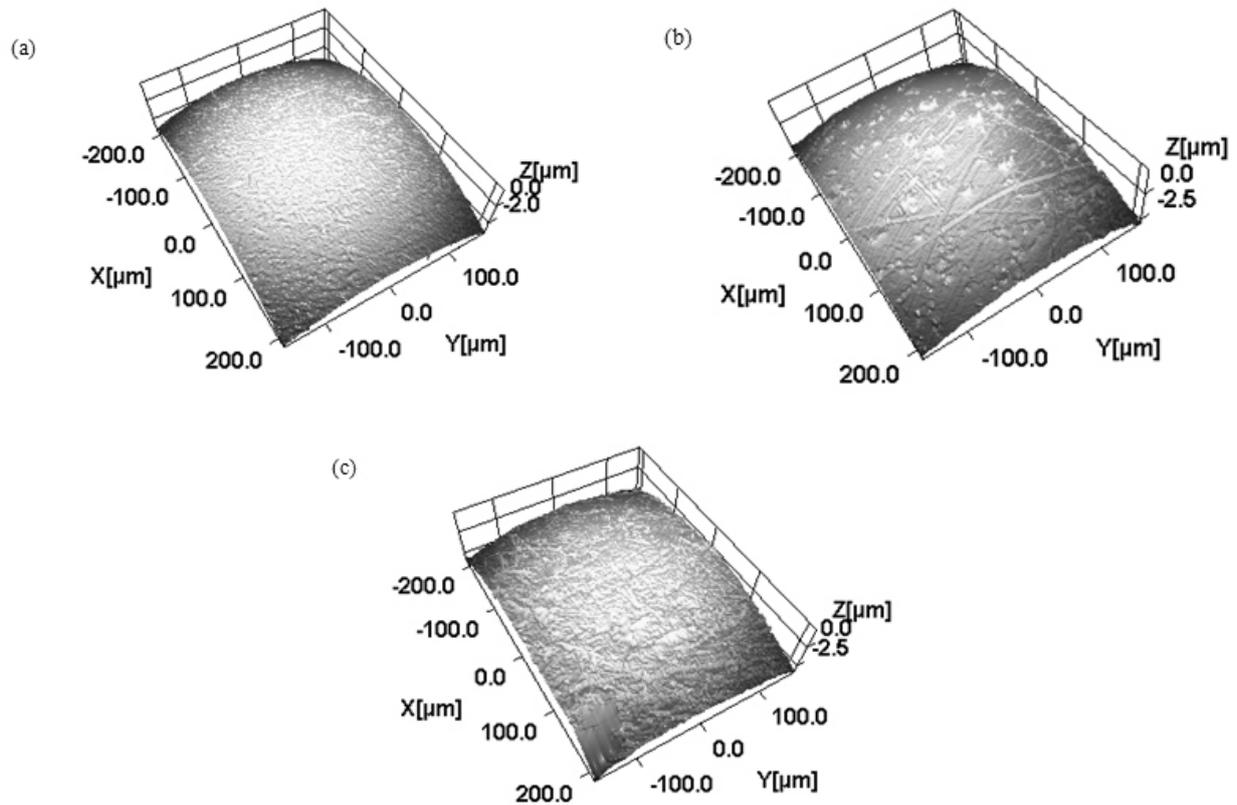
**Fig. 2.** 3-D optical profile of (a) 440C stainless steel (b) Al alloy (2017) (c) bronze ball counterface.
