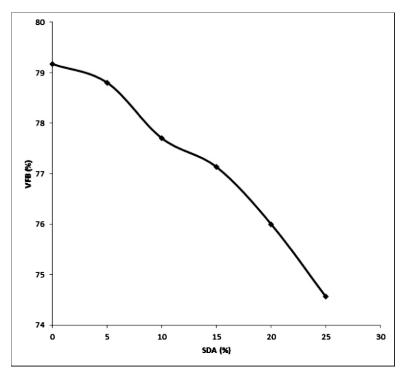
Figure 5: Variation of Voids Filled with Bitumen (VFB) with Increasing Sawdust Ash (SDA) in the Asphaltic Concrete
