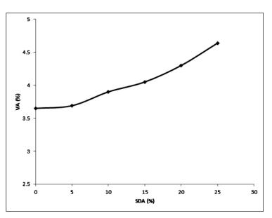
Figure 6: Variation of Air Voids (VA) with Increasing Sawdust Ash (SDA) in the Asphaltic Concrete
