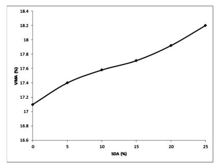
Figure 7: Variation of Voids in Mineral Aggregate (VMA) with Increasing Sawdust Ash (SDA) in the Asphaltic Concrete
