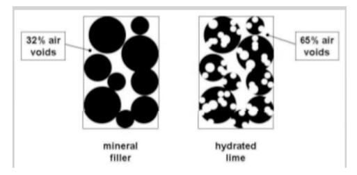
Figure 3: Porosity of Granite and Hydrated Lime Filler Particles Source: Lesueur*et al.* (2012)
