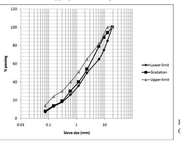
Figure 1: Aggregate Gradation Curve
