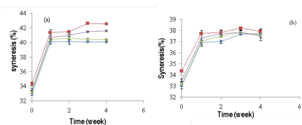
Figure 4: Syneresis and freeze thaw stability study of native maize starches of at -15°C (a) and 4°C (b).
