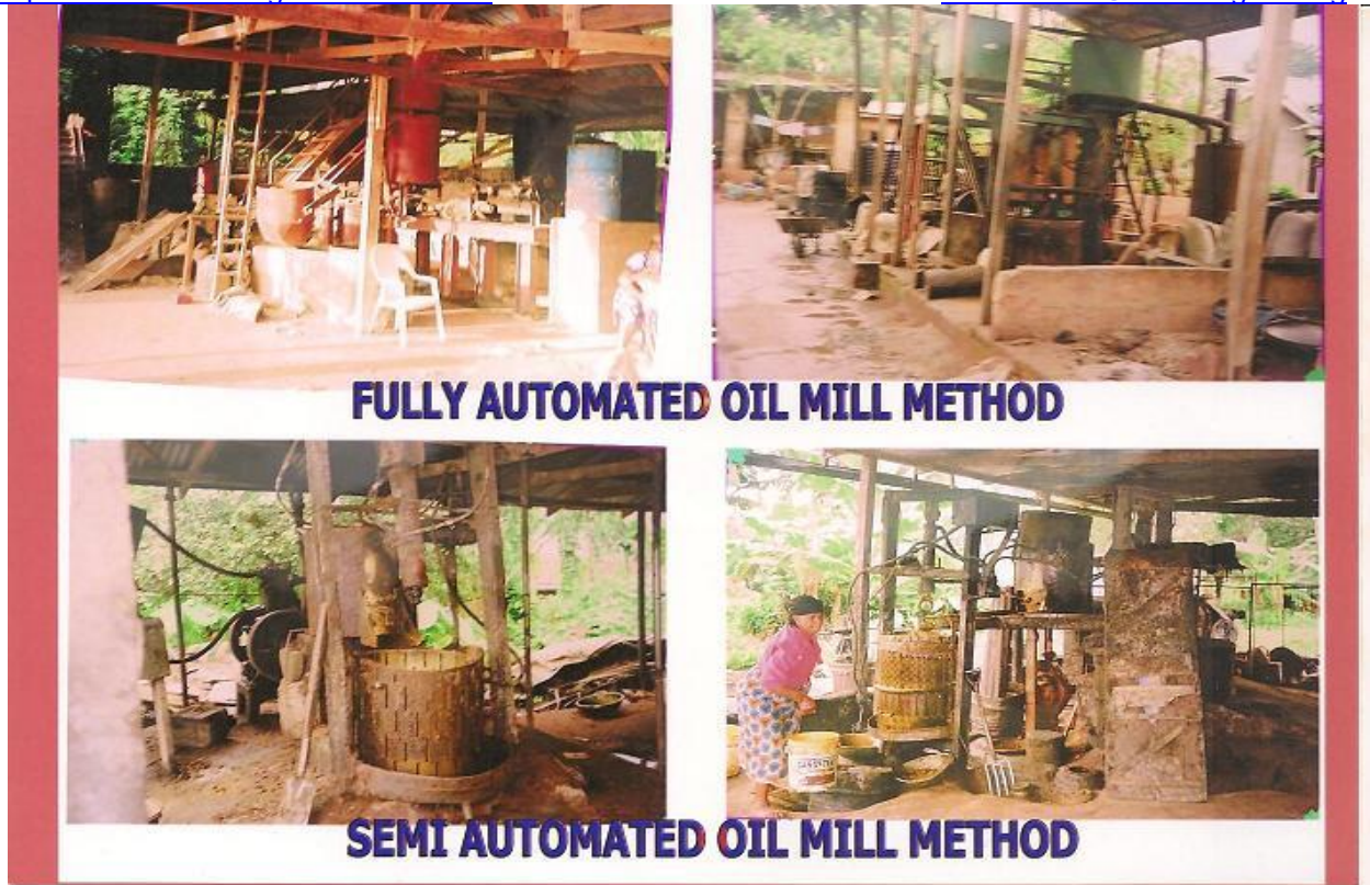
Plate 1(a): Fully automated oil mill comprising of sterilizer, digester, press, fibre separator and oil clarification. (b) Semi automated oil mill comprising cooking drums, digesters, press, manual fibre separation and oil clarification
