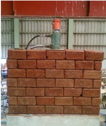
Figure 1: Typical arrangement of wall model for testing
