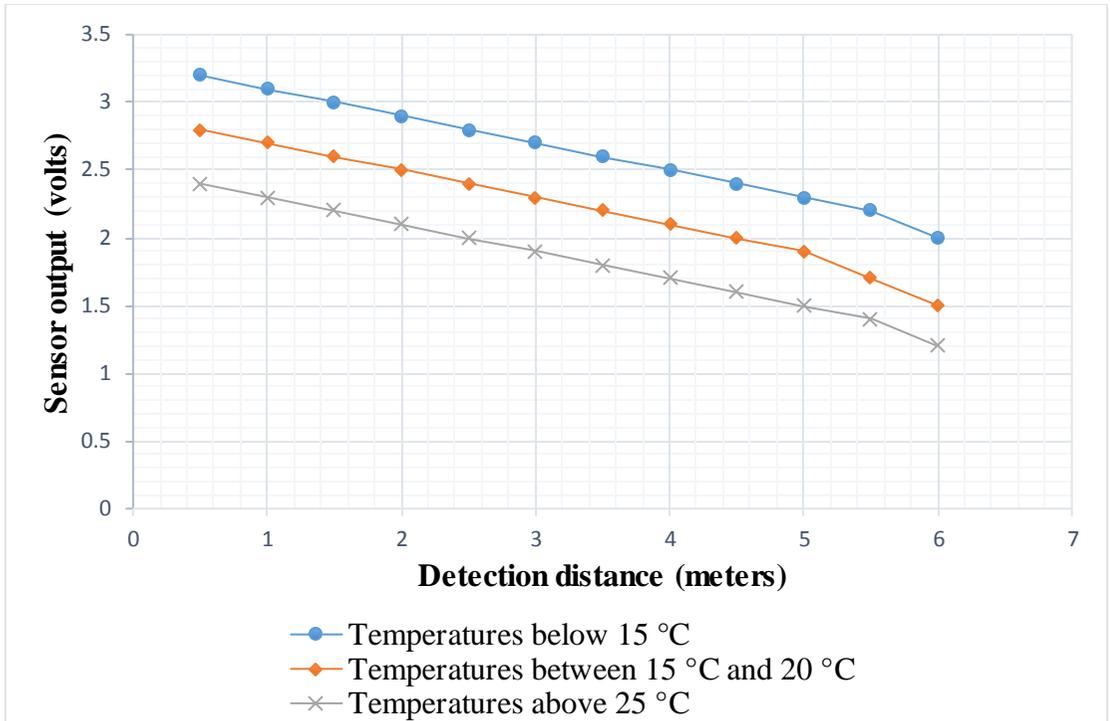
Fig. 3: A graph of sensor output against detection distance showing the inverse relationship between temperature and PIR sensor sensitivity.
