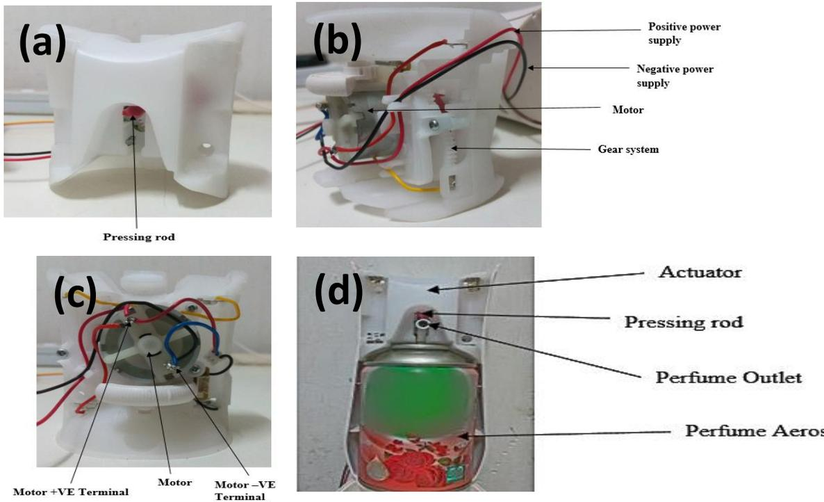
Fig. 2: (a) Front view, (b) Side view (c) Back view and (d) the actuator system and aerosol containing rose fragrant perfume fitted in the actuator element.
