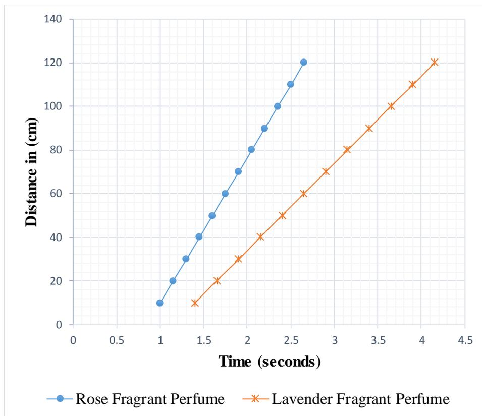
Fig. 6: A plot of distance (cm) against time (seconds) on using MQ2 Detector measured at temperatures of 29°C for Rose and Lavender Fragrant Perfumes.
