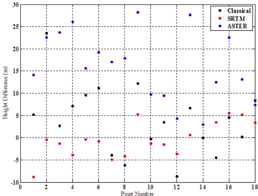
Fig. 1: differences between levelled and DEM orthometric heights
