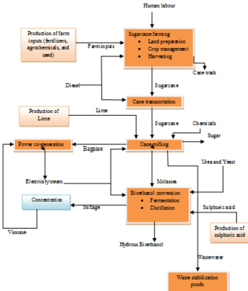
Figure 1: System boundary for sugarcane molasses based bioethanol
