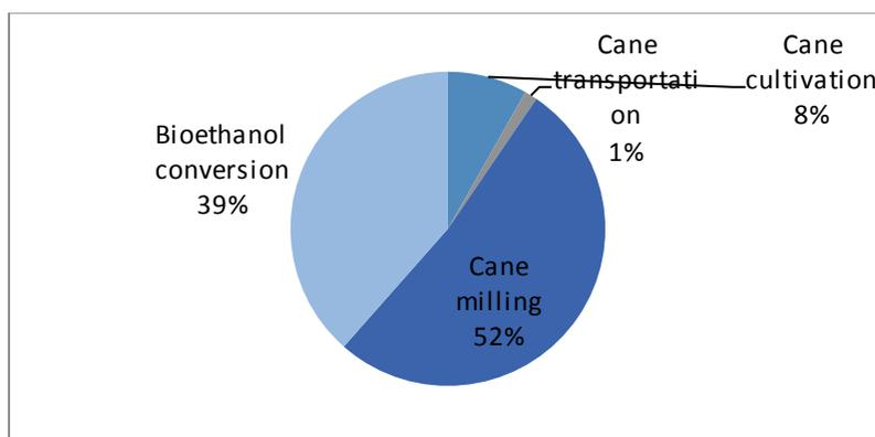
Figure 3: Energy consumption for sugarcane molasses based bioethanol in Kenya
