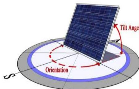
Figure 1: Tilt angle of a solar panel (Al-Ghamdi & Alshaibani, 2018).
