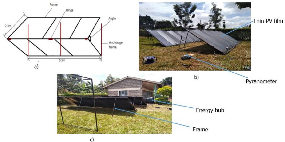
*Figure 4: Thin-film PV system tilt angle set-up.*
