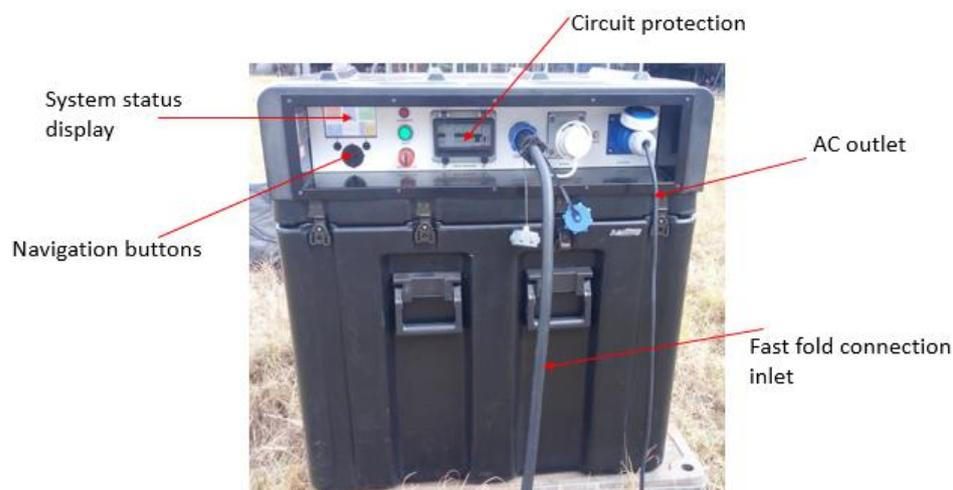
Figure 3. Fast fold energy hub
