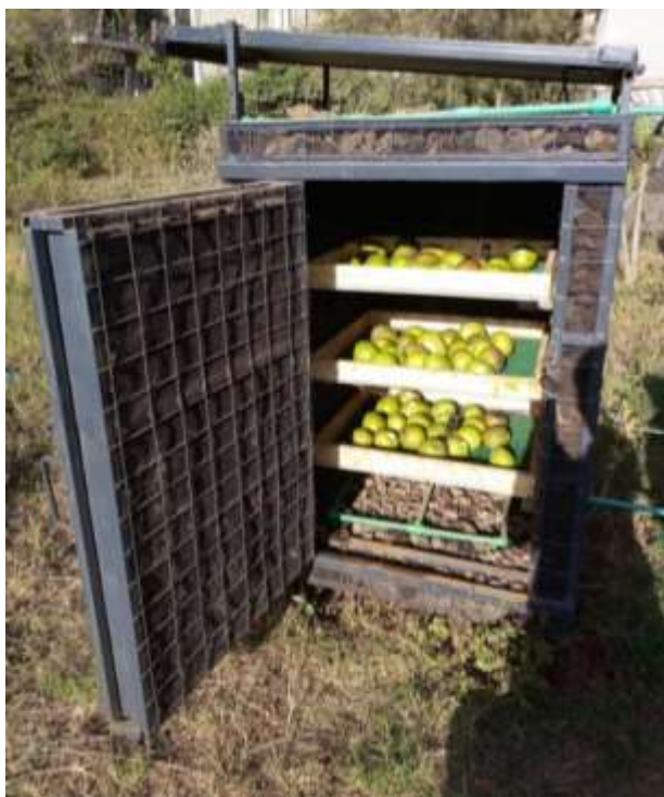
Figure 4: shows the developed cooler loaded with mangoes at the beginning of an experiment to determine the effect of storage environment on quality of the fruit
