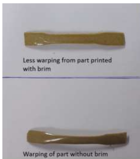
Figure 4: Image showing the difference in the prints when a brim is included
