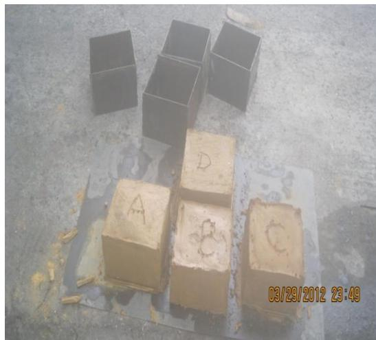
**Fig. 1:** Moulded samples and metallic moulds
