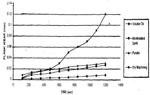
Fig.3: Graph of flank wear (mm) against t (sec) with high speed steel cutting tool and mild steel workpiece
