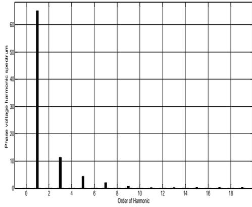
**Fig. 13.** Phase voltage harmonic component. (THD=16%)
