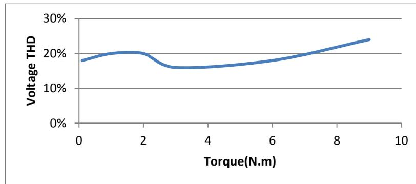
**Fig 19.** Variation of Voltage THD due to Torque
