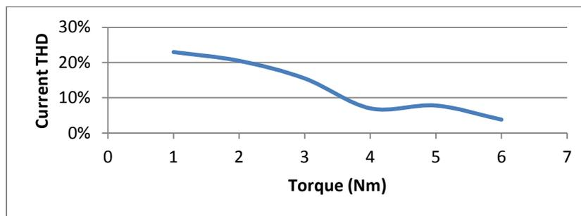
**Fig 20.** Variation of current THD due to Torque
