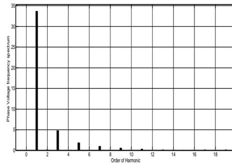
**Fig. 10.** Harmonic component of output voltage.(THD=16%).
