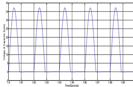
**Fig.8.** Voltage of Capacitor<sub>2</sub> (Converter A)
