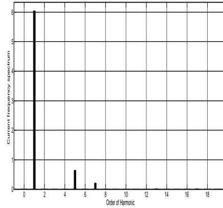
**Fig. 14.** Line Current Harmonic Component. (THD=7%)
