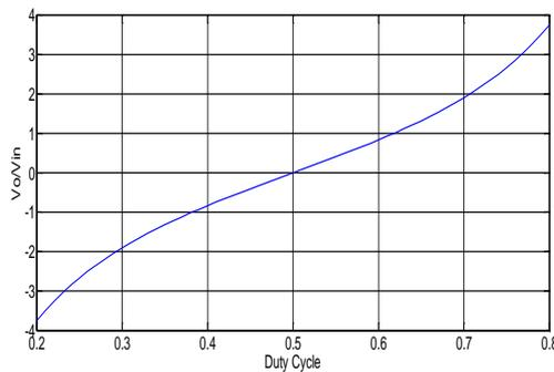
Fig. 6: Dc gain characteristic.
