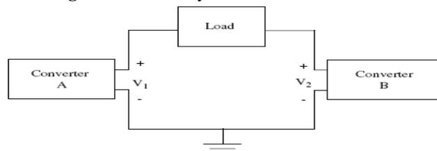
**Fig. 3.** Basic approach to achieve dc-ac conversion, with boost characteristics
