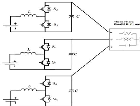
Fig. 5. The boost three phase inverter used in the proposed scheme.
