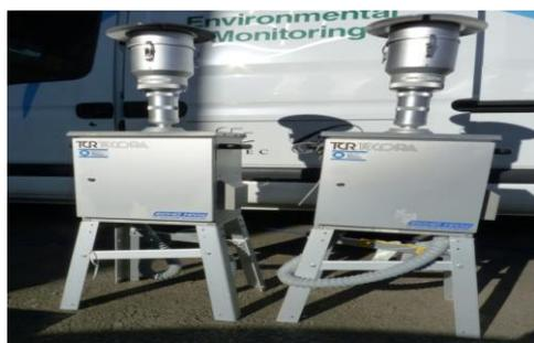
**Fig 1.** Tecora Echo high volume PM<sub>10</sub> sampler.
