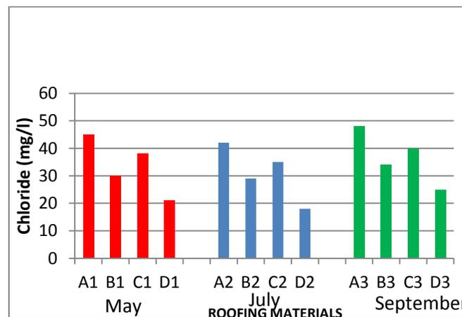
**Fig 5:** Chloride concentration of rainwater harvested from different roofing materials
