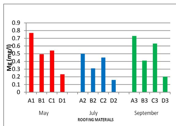
**Fig 9:** Magnesium concentration of rainwater harvested from different roofing materials A = Asbestos, B = Aluminum, C = Zinc, D = Control
