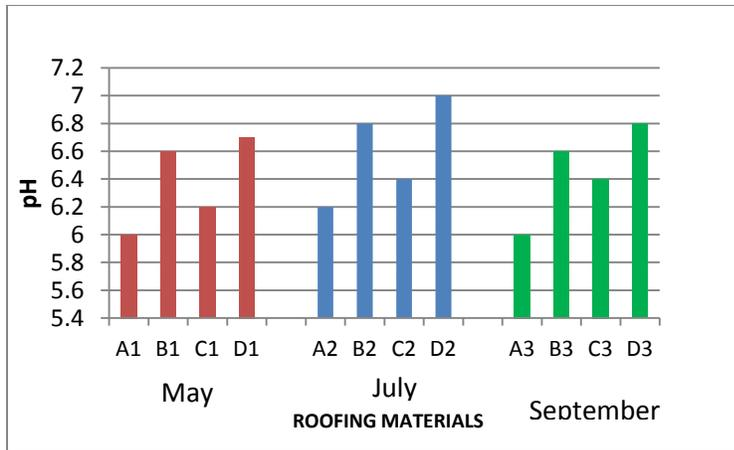
**Fig2:** pH concentration of rainwater harvested from different roofing materials
