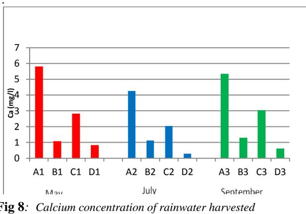
**Fig 8:** Calcium concentration of rainwater harvested from different roofing materials A = Asbestos, B = Aluminum, C = Zinc, D = Control
