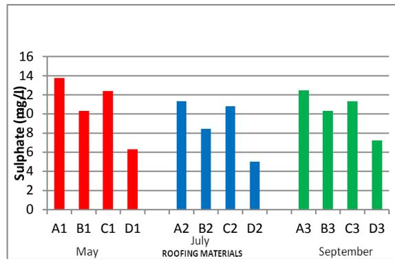
**Fig 7:** Sulphate concentration of rainwater harvested from different roofing materials A = Asbestos, B = Aluminum, C = Zinc, D = Control
