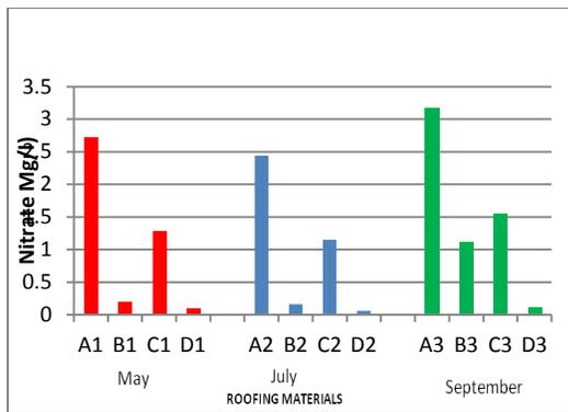
**Fig 6:** Nitrate concentration of rainwater harvested from different roofing materials A = Asbestos, B = Aluminum, C = Zinc, D = Control
