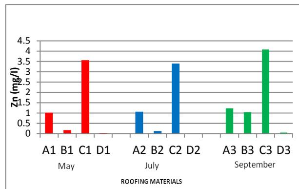
**Fig 11:** Zinc concentration of rainwater harvested from Different roofing materials A = Asbestos, B = Aluminum, C = Zinc, D = Control
