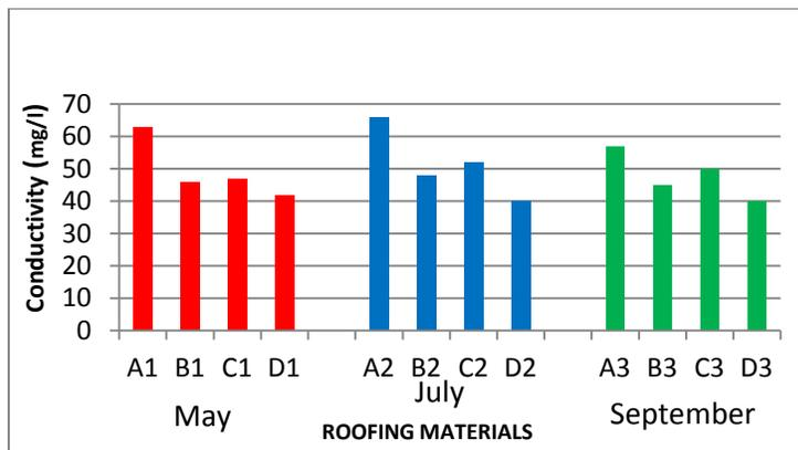
**Fig 3:** Conductivity concentration of rainwater harvested from different roofing materials
