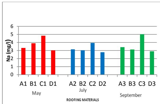
**Fig 10:** Sodium concentration of rainwater harvested from different roofing materials A = Asbestos, B = Aluminum, C = Zinc, D = Control
