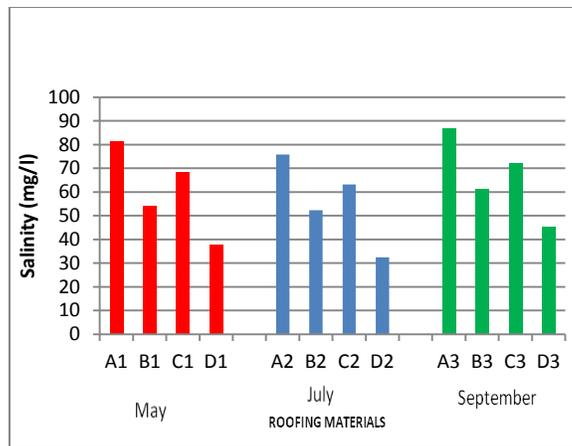
**Fig 4:** Salinity concentration of rainwater harvested from different roofing materials
