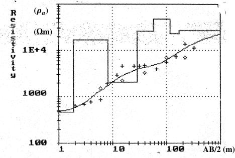
Fig 2: Typical Sounding Curve for Ejeme-Aniogor and Environs (VES 1)
