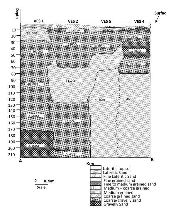
Fig 5: Geoelectric section of the VES results (VES 1,2,4 and 5)
