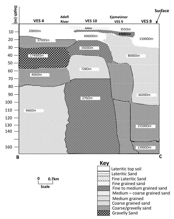
Fig 6: Geoelectric Section of the VES results (VES 4,8,9,10)
