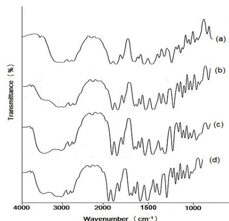
**Fig 2:** FTIR spectra of pure acetylsalicylic acid crystals (a) and the tablet granules prepared with pre-gelatinized starches of bitter yam (b), cassava (c) and maize (d)
