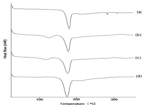
**Fig 1:** DSC thermograms of pure acetylsalicylic acid crystals (a) and the tablet granules prepared with pre-gelatinized starches of bitter yam (b), cassava (c) and maize (d)
