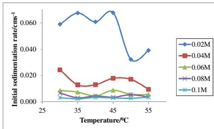
Fig 2: Initial sedimentation rate of TCP precipitate as function of temperature for various  $[PO_4^{3-}]$ .
