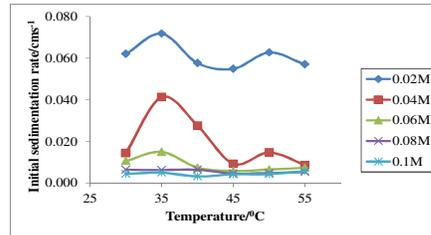
Fig 4: Initial sedimentation rate of TSP precipitate as function of temperature for various  $[PO_4^{3-}]$ .
