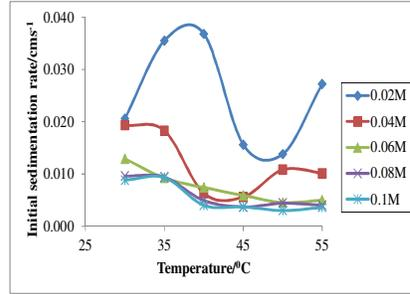
Fig 3: Initial sedimentation rate of TSP precipitate as function of temperature for various  $[Sr^{2+}]$ .
