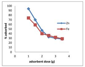
Fig 3: Effect of adsorbent dose on adsorption of Zn and Fe onto activated carbon
