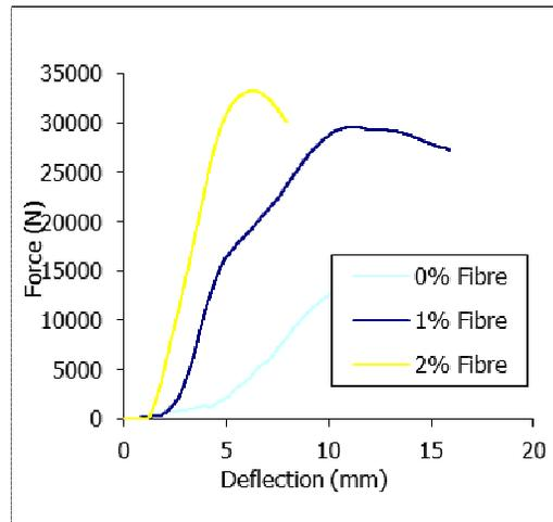
Fig 7: Load vs Deflection Curve for carbon fibre
