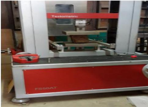
Fig 5: Compressive strength test using the Testometric machine
