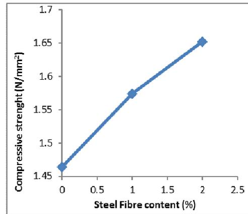
Fig 10: Influence of steel fibre content on compressive strength
