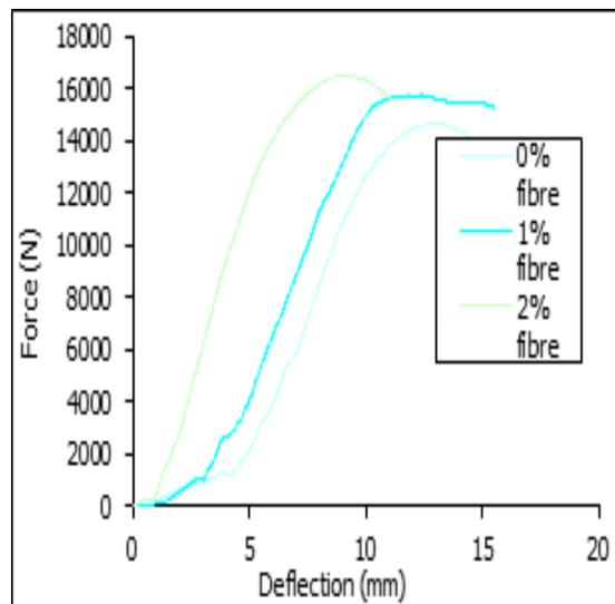
Fig 11: Load-deflection curve for steel fibre
