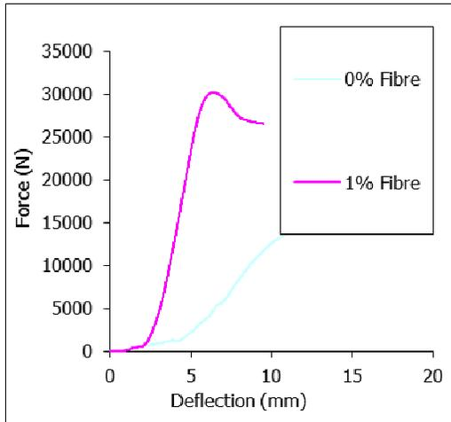
Fig 9: Load - Deflection curve for palm kernel fibre
