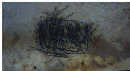
Fig 3: Steel fibres
