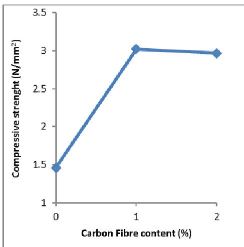
Fig 6: Compressive Strength (N/mm<sup>2</sup>) against Carbon fibre content (%)
