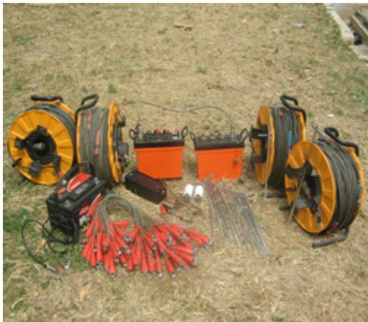
**Fig 4.** ABEM LUND Imaging System together with Terrameter SAS 4000 and ES 464 used for Electrical Resistivity Tomography
