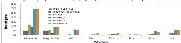
Fig 1: Comparative level of metallic content of NPO, NPeO, NSPO, NSPeO with EN 14214 and ASTM D 6751 standard. NPO, Nigerian palm oil; NPeO, Nigerian peanut oil; NSPO, Nigerian spent palm oil, NSPeO, Nigerian spent peanut oil.
