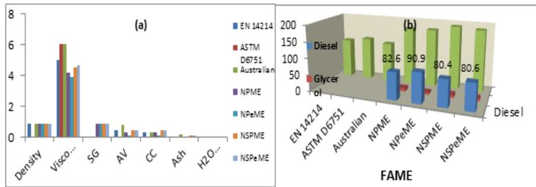
**Fig 3:** Biofuel properties (a) and Yield of biodiesel, glycerol and FP (b) of NPME, NPeME, NSPME, and NSPeME after two steps alkali transesterification. NPME, Nigerian palm methyl ester, NPeME, Nigerian peanut methyl ester, NSPME, Nigerian spent palm methyl ester, and NSPeME, Nigerian spent peanut methyl ester.
