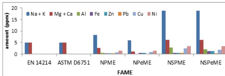
**Fig 4:** Level of metals in NPME, NPeME, NSPME, NSPeME after two steps transesterification.
