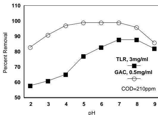
Fig 1. Effect of pH on COD removal
