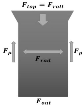
Fig 1: The forces acting in the pellet channel.
