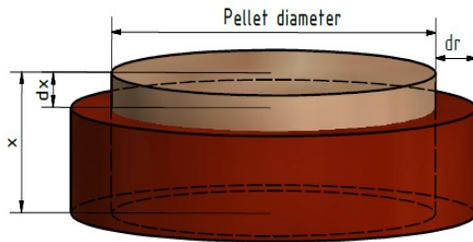
Fig 2: Compression of an element in the 1D model, causing a radial expansion.
