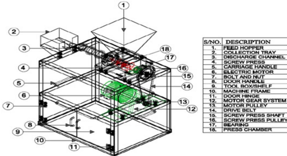
Fig 3: Skeletal view of the pelleting machine
