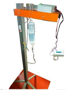
Fig 7: Automated alert system of an intravenous infusion system
