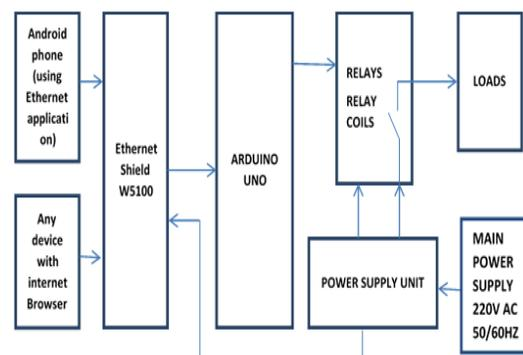
Fig 2: Schematics of smart switch system
