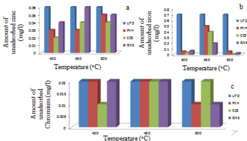
Fig 7. Concentration of un-adsorbed (a) Zn (b) Fe (c) Cr metal using PKH, CCS, and GNS activated with 0.2 M ZnCl<sub>2</sub> and untreated (UTD) wastewater
