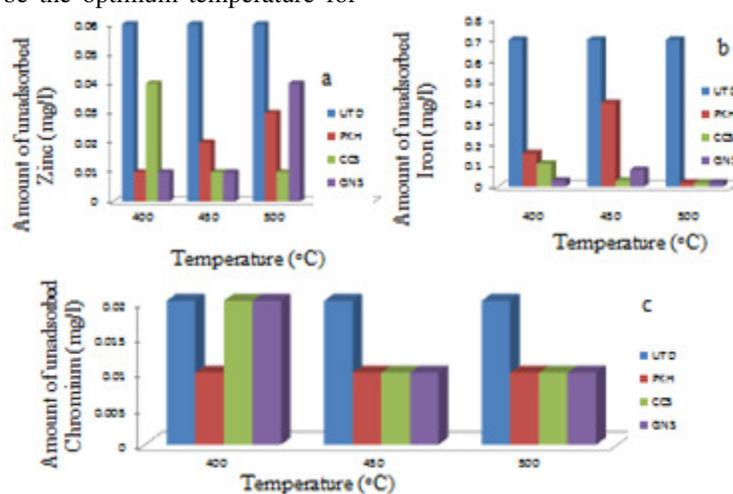
**Fig 5:** Amount of un-adsorbed (a) zinc (b) iron (c) chromium 0.2 M KOH with palm kernel husk (PKH), coconut shell (CCS), groundnut shell (GNS) as adsorbent and untreated (UTD)
