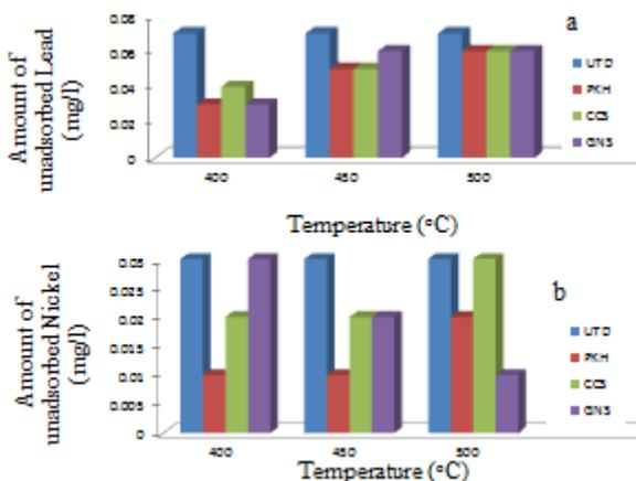
Fig 4: Amount of un-adsorbed (a) lead (b) nickel 0.2 M KOH with palm kernel husk (PKH), coconut shell (CCS), groundnut shell (GNS) as adsorbent and untreated (UTD)
