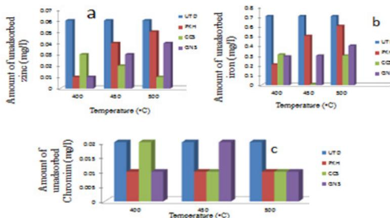
**Fig 1.** Amount of un-adsorbed (a) zinc (b) iron (c) chromium for 0.1 M KOH with palm kernel husk (PKH), coconut shell (CCS), groundnut shell (GNS) as adsorbent and untreated (UTD)
