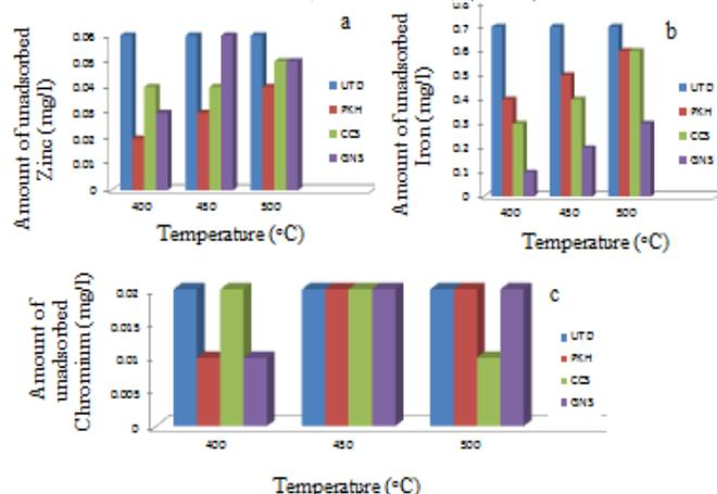
Fig 3: Amount of un-adsorbed (a) zinc (b) iron (c) chromium for 0.2 M KOH with palm kernel husk (PKH), coconut shell (CCS), groundnut shell (GNS) as adsorbent and untreated (UTD)
