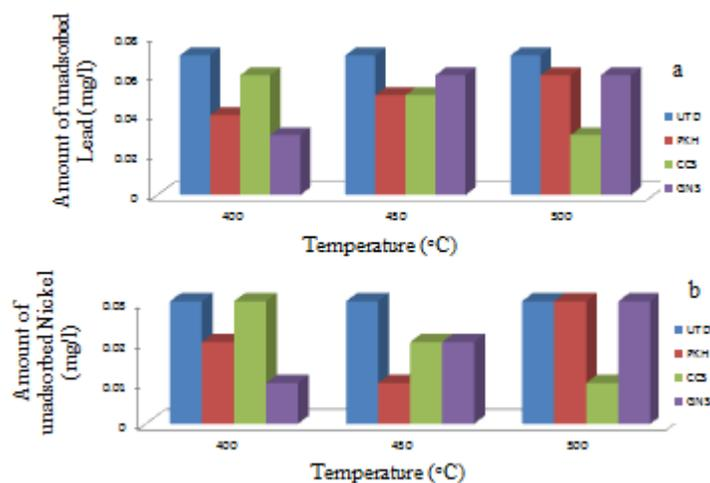
**Fig 8.** Concentration of un-adsorbed (a) Pb (b) Ni metal using PKH, CCS, and GNS activated with 0.2 M  $ZnCl_2$  and untreated (UTD) wastewater
