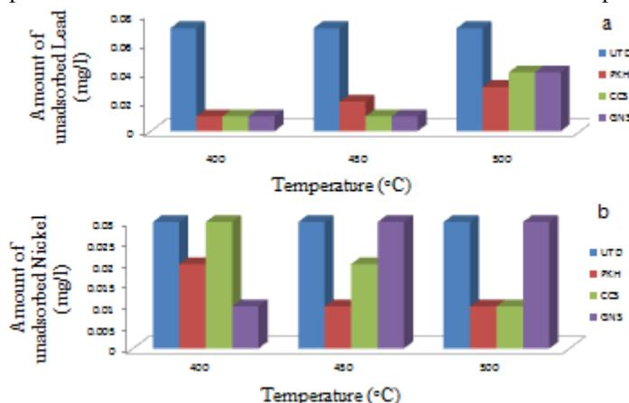
Fig 6: Concentration of un-adsorbed (a) lead (b) nickel metal using palm kernel husk (PKH), coconut shell (CCS), groundnut shell (GNS) activated with 0.1 M ZnCl<sub>2</sub> as adsorbent and untreated (UTD) waste-water
