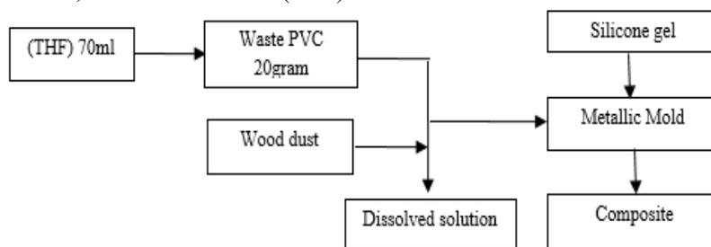
Fig 1: Schematic view of production procedure
