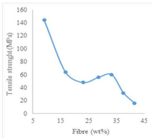
Fig 2: Tensile strength of composite at different weight percent
