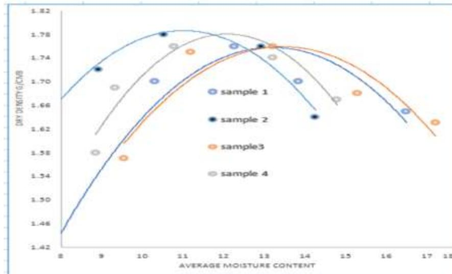
Fig 3: Compaction curves
