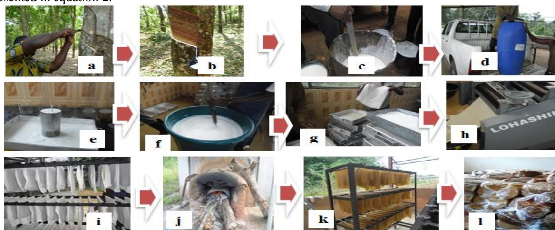
Fig 1. Field latex processing into ribbed smoked sheets in RRIN (Images; a - tapping of rubber tree, b - collection of NR latex, c - bulking of field latex, d- transportation of field latex to the processing factory, e- determination of DRC with metrolac. f- Dilution of latex and
