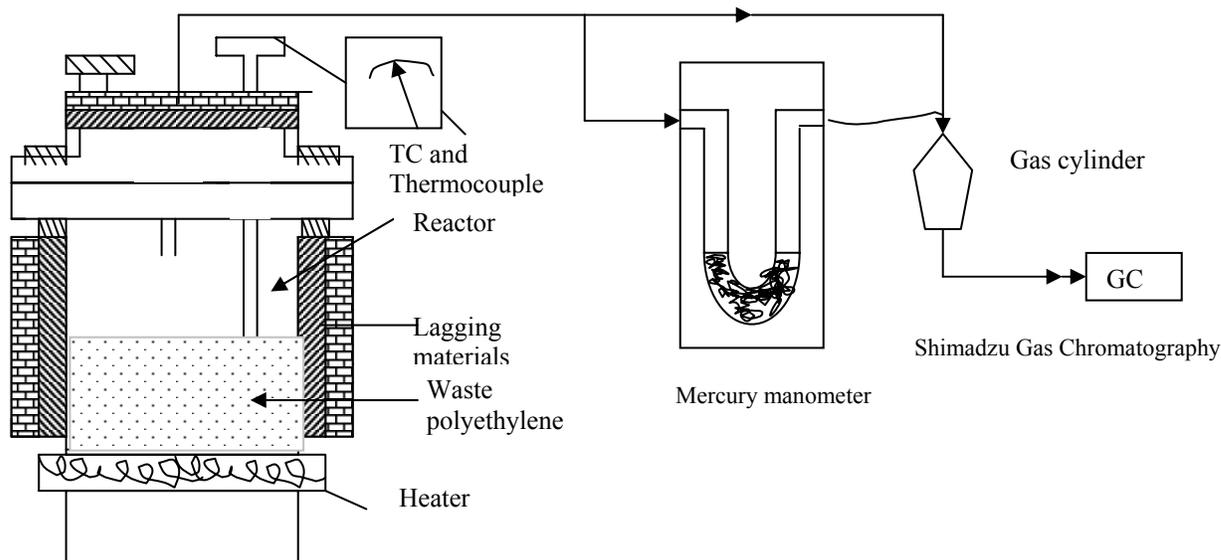
**Fig 1.** Reactor for pyrolysis
