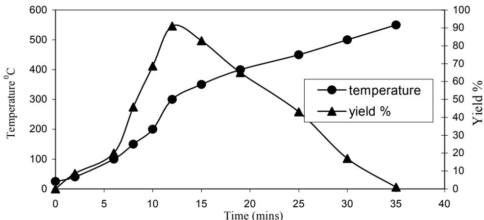
Fig 3 Effect of Temperature and time on the yield of gaseous products
